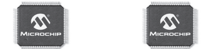
PF: 80引脚TQFP (14 x 14 x 1 mm) P: 100引脚TQFP (14 x 14 x 1 mm)
